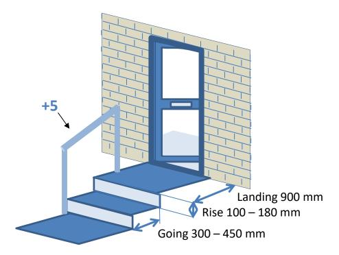
Single steps or short flights between rooms, in circulation spaces or at thresholds are hazardous and should be avoided, so that Internally all the rooms on each storey should be accessible without the need to use steps. If steps are unavoidable, then their presence should be clearly discernible through contrasting floor finishes and a handrail, even on single steps.
