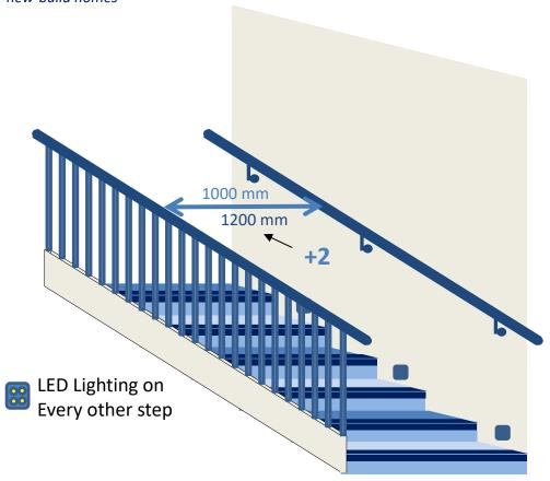
Two graspable handrails. The clear width between handrails to be a minimum of 1000 mm. Install LED lighting such that every other step is illuminated providing contrast between steps. Nosings should contrast visually (distinguishable difference in light reflectance value, around 30 points, as measured using BS 8493:2008+A1:2010) with the rest of the tread through added material which is 50-65 mm on the tread and 30-55 mm on the rise.
