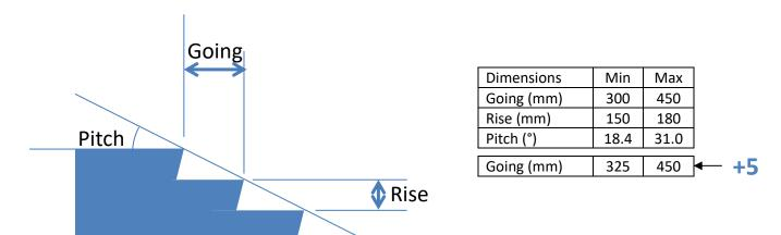
Going and rise are measured nosing to nosing. Values in tables are nominal, with 1% tolerance allowed. Hence measured going on any step could be  $300 \text{ mm} \pm 3 \text{ mm}$ .
