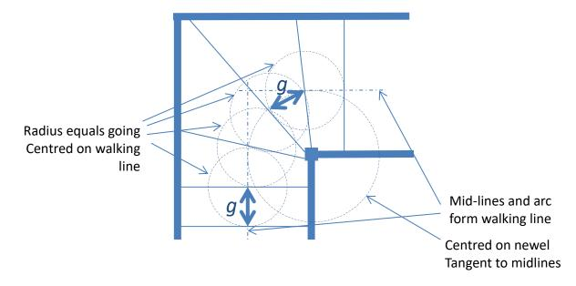
By considering the winders first, and using these construction rules it is possible to make the goings on winders equal to the goings on the straight parts of any stair. Note at the newel post nosings must be a minimum of 50 mm apart.
