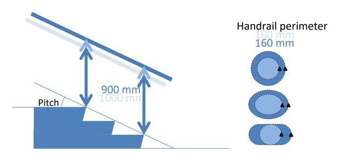
Handrail to be parallel to the pitch line and the top of the handrail to be between 900 mm and 1000 mm vertically above the pitch line.
