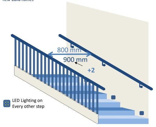
Add a second handrail, and ensure at least one of them is graspable. Clear width between handrails (or handrail and guarding if only one handrail) to be a minimum of 800 mm. Install LED lighting such that every other step is illuminated providing contrast between steps.
