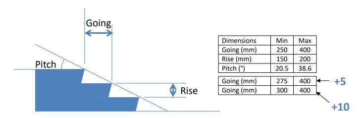
Going and rise are measured nosing to nosing. Values in tables are nominal, with 1% tolerance allowed. Hence measured going on any step could be 250 mm ± 2.5 mm.
