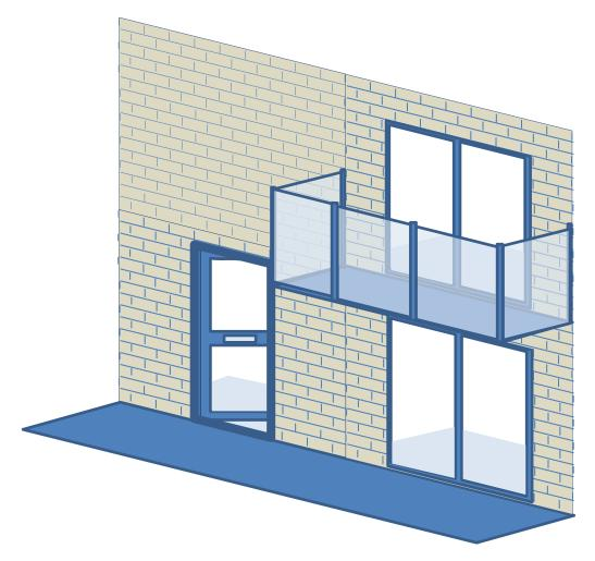
To be step free for this document, every entrance into the dwelling must be accessible without the need to use steps including balconies and patio doors. The external ground level or balcony surface should therefore be at the same height as the internal floor level adjacent to it.
