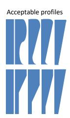
Suitable step profiles should be closed risers with an overlap between 0 mm and 25 mm. Profiles may be square or curved. The rake must be 60° or steeper, and therefore rise through a height of between two times the overlap and the full height of the riser. A number of alternative shapes may be acceptable, however consideration should be given to the shape of available proprietary nosings before choosing a particular profile.
